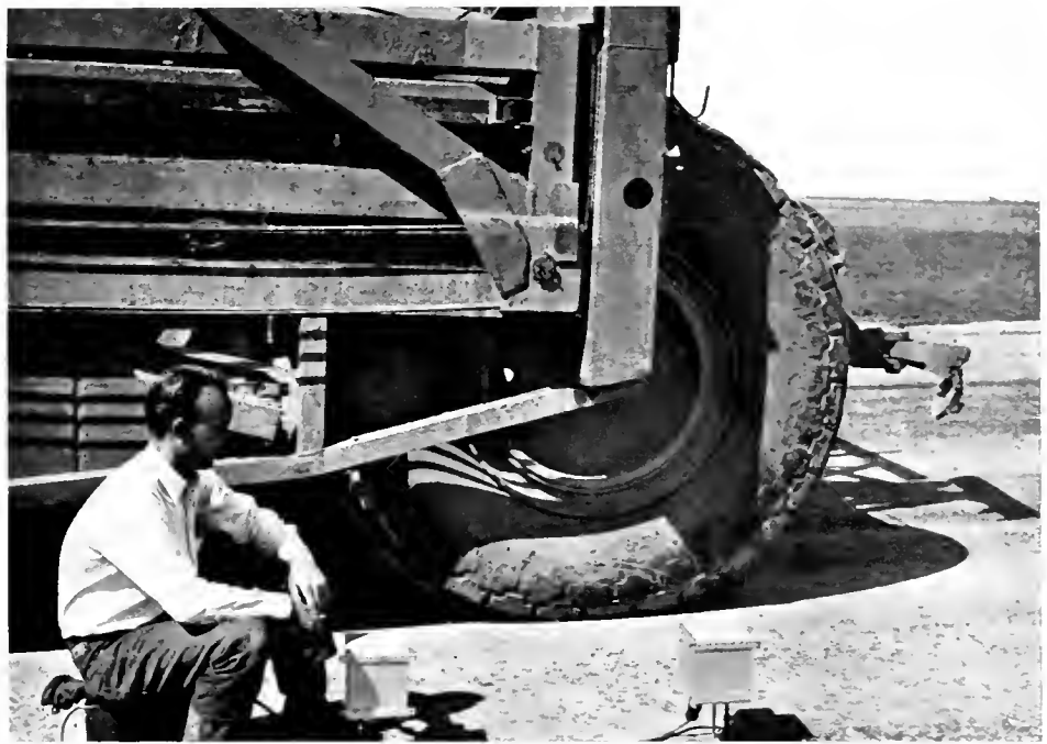
Determining deflection of pavement under loads corresponding in footprint and contact pressure to those of heavy bombers. Electric eye equipment in boxes in foreground
